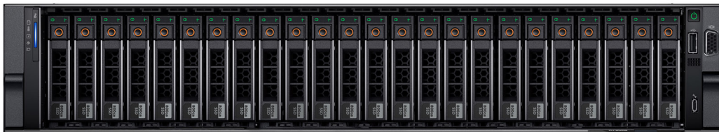
Figure 1. Front view of 24 x 2.5-inch drive system
