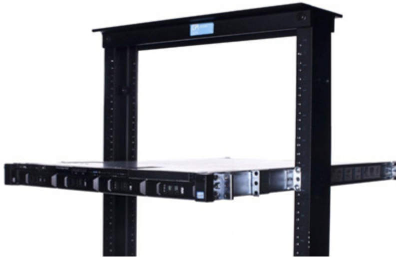
Figure 28. Static rails in 2-post center mount configuration
